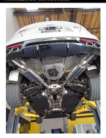
**Step 4:** Once a final position has been chosen for the new exhaust system, evenly tighten all clamps from front to rear using the torque specifications on page one of these instructions. Tighten fasteteners for Muffler brace and install factory underbody brace. Inspect all fasteners after 25-50 miles for operation and re-tighten if necessary.
