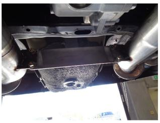
**Step 3:** Next Install the Muffler Assemblies to the outlets of the Resonator Assembly using the supplied 2.50" clamps. Insert hangers into rubber insulators. At this time loosely attach the Magnaflow logo brace to tie the muffler assemblies together using the supplied fasteners.
